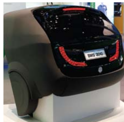
An all-polycarbonate tailgate prototype by Bayer MaterialScience opens up new styles and moulding options
