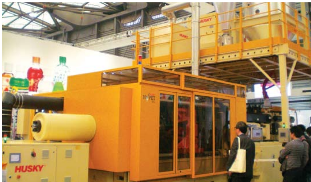
Husky's HyPET HPP system produces preforms containing up to 50% post-consumer PET flakes
