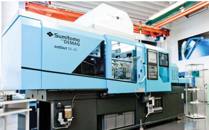
The IntElect injection moulding machine by Sumitomo (SHI) Demag tackles micro POM parts for hearing aid devices
