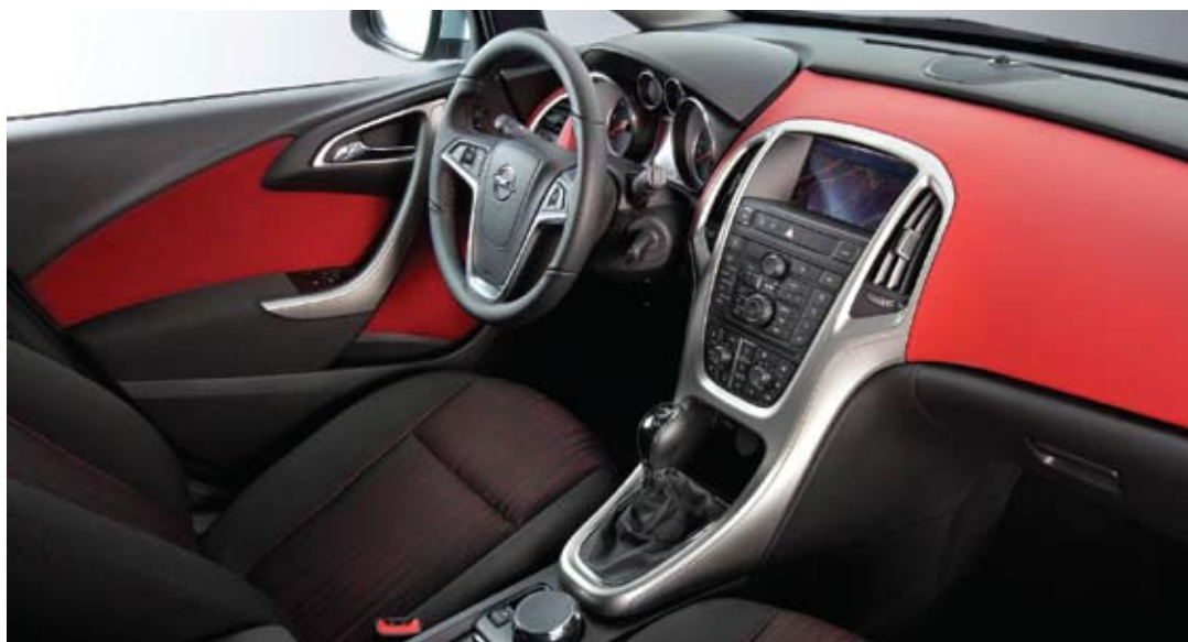
LyondellBasell's Softell PP compound is used for instrument panel, the B and C pillars and the door panels of the recently launched new Opel Astra model
