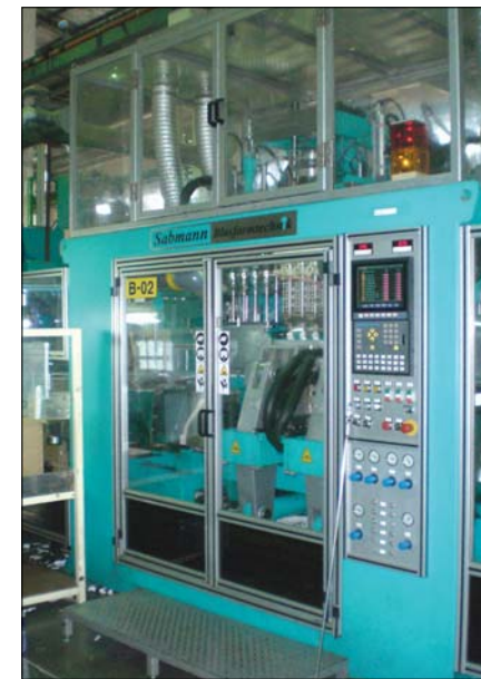
Co-extrusion blow moulding processes are a key part of Dynaplast Packaging's production operations in Vietnam
