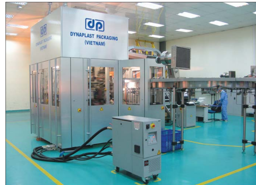
Dynaplast Packaging Vietnam installed an inline stretch injection stretch blow moulding line at one of its customer's premises for PET bottling production and filling
